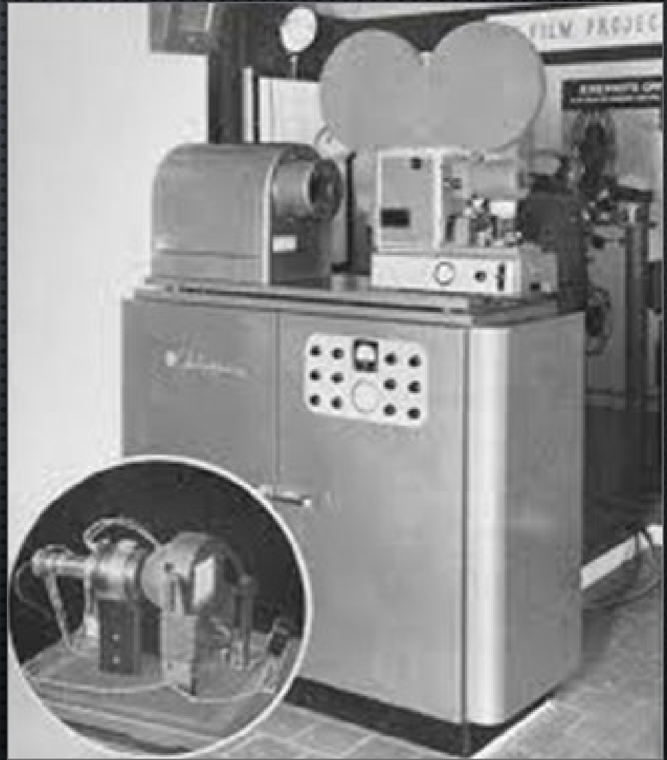
RCA Kinescope for recording TV programs on film, 1953
